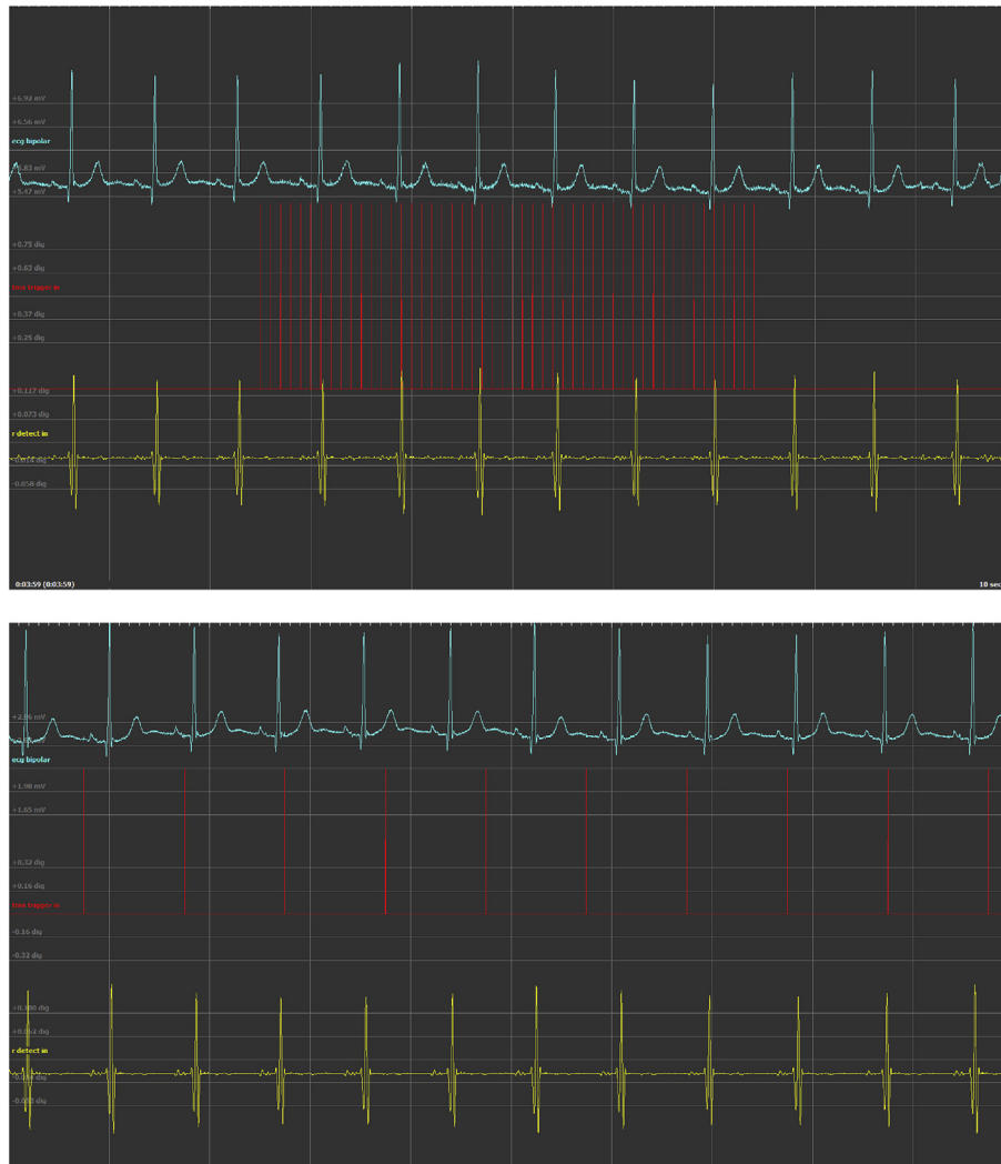
Fig. 1. An example of high-frequency NCG-TMS (top) and low-frequency NCG-TMS (bottom) data with the ECG trace represented in blue, the TMS triggers represented in red and the R-peak detection by the NCG-TMS module in yellow. (For interpretation of the references to colour in this figure legend, the reader is referred to the Web version of this article.)
